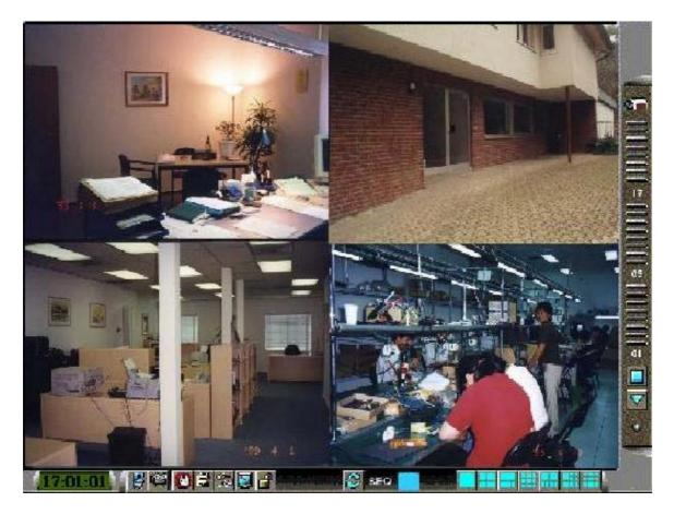
The diagram above is the main screen display. The icons on the lower corner of the screen are mainly for control and configuration, those on the right corner for status indication. If any icon is grayed, it means that the specific function is not accessible in the current mode or login right.
